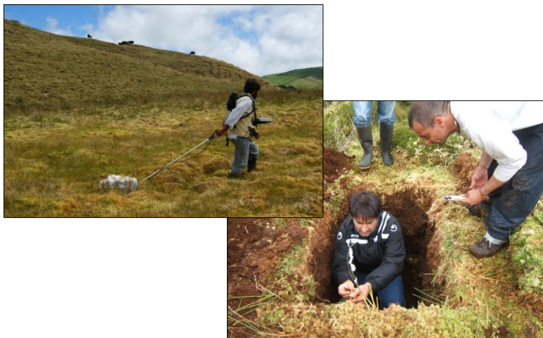
Georadar and Coring
